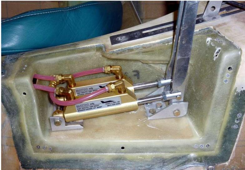
Fig 10. Platform / Master Cylinder sub-assembly (inlet ports point aft due to throttle spine removal)
