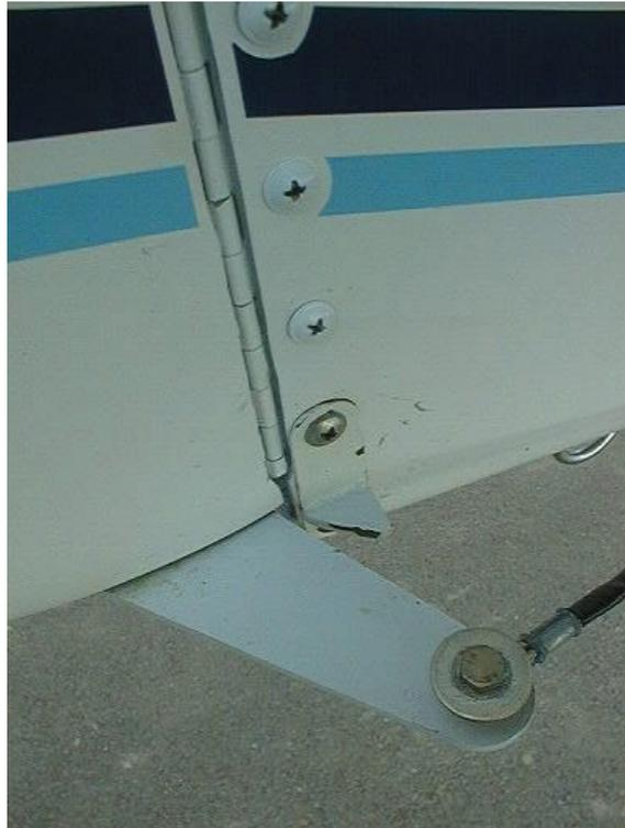
*Fig 10. Photo of starboard rudder stop.*
